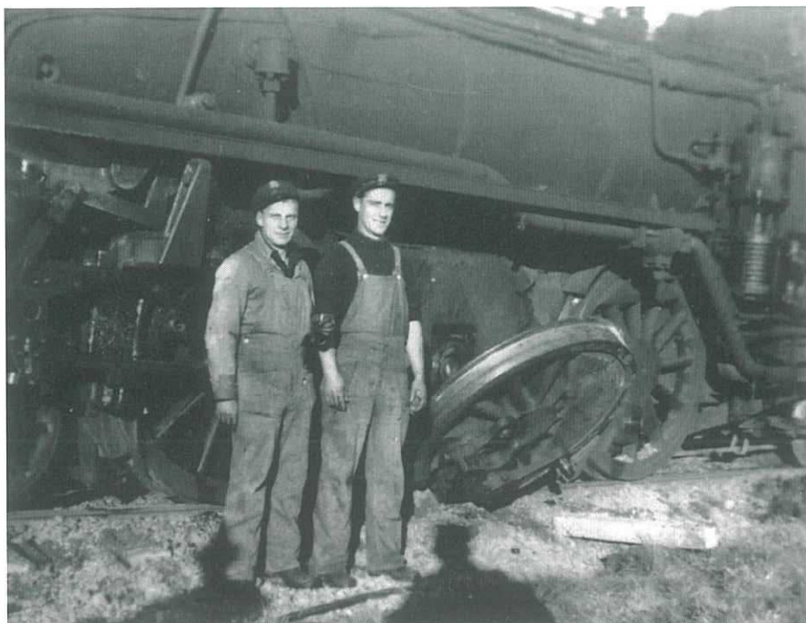
Bob Carson and Jack Knight with AB696 and a broken axle on the main driving wheel while climbing the Dashwood Pass, c.1950
